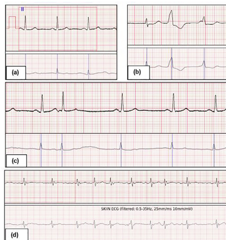
Figure 1 - ECG measured by the gold standard system with gel at the chest (Standard ECG, Lead II, top) and Skiin underwear band at the waist (pseudo-Lead I, bottom) during: (a) sinus rhythm, (b) Premature Ventricular Contractions, (c) Premature Atrial Contractions, and (d) Atrial fibrillation.
